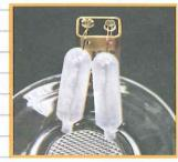
8. Connect the other ends of the paper clips to the two poles of the battery. The process of electrolysis starts.
